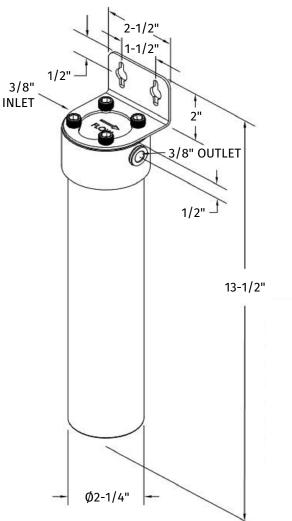
MINIMUM 11" REQUIRED BETWEEN BOTTOM OF CANISTER AND BOTTOM OF CABINET FOR CARTRIDGE REPLACEMENT
